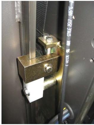
3. Align the limit switch on the inside of the tower with the center of the strap.
